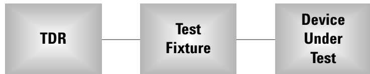
Figure 3. Test system with the device at the end of an imperfect test fixture.
